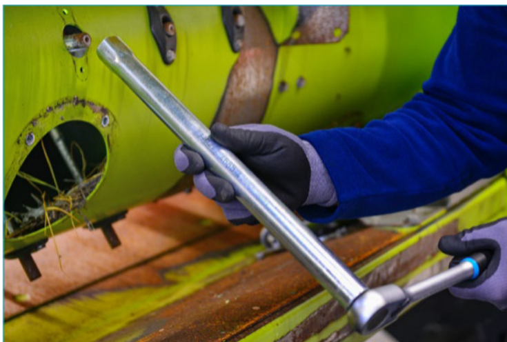
Operating using ratchet with inserted 12.5 mm (1/2") 4-point socket
