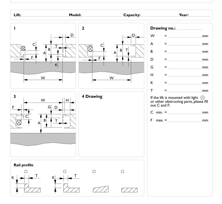
PLEASE NOTE: It is the customer's responsibility that the given measures are correct and sufficient. The lift shall always be approved by the lift manufacturer for mounting of jacking beams. N.b. EN1493:1998 the capacity of the jacking beam cannot exceed 0,66 x the capacity of the lift. (A 2 t jacking beam on a 3 t lift is okay - but not a 2,6 t).
