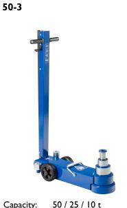
Capacity: 50 / 25 / 10 t Max. height: 210 / 265 / 335 mm
